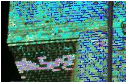
Material identification is possible with the hyper-spectral imagery by analyzing the molecular response spectrum. Image by Zohreh Zahiri, PhD
