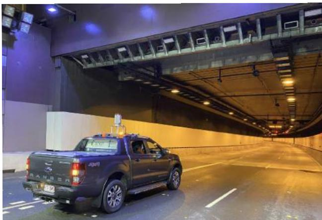
The vehicle-mounted RIEGL VZ-400 terrestrial laser scanner allows Orion the flexibility to move around obstacles, and stop and start as needed. Image by Orion
