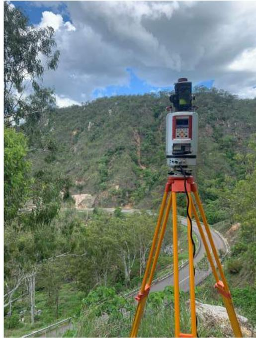
RIEGL VZ-400 terrestrial laser scanner in action at the Australian mine. Image by Orion.
