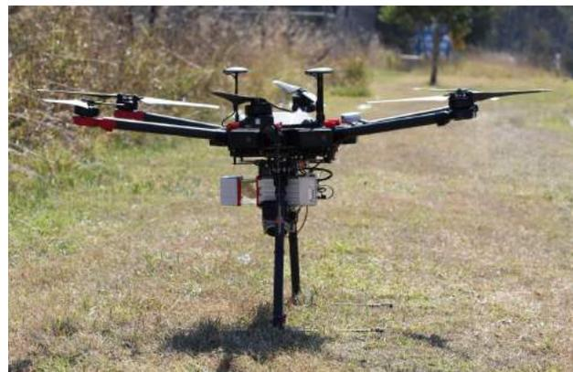
ABOVE: A RIEGL miniVUX-2UAV unmanned LiDAR scanner mounted on the M600 UAV platform gave crews the ability to fly over the rugged terrain. Images by Orion.
